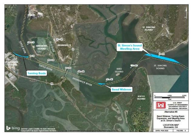
Figure 6 - Alternative 8 Bend widener, turning basin expansion, and meeting area at St. Simons Sound
